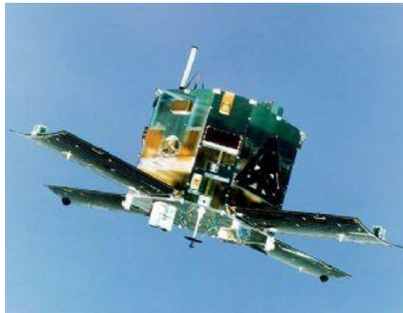
Figure 4: Locations of 4 electrodes which are attached at the ends of solar cell panels.
