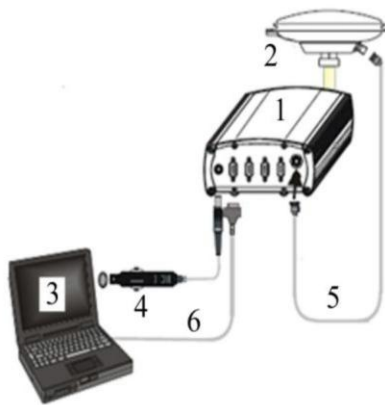
Figure 1. Hardware-software complex of monitoring ionosphere: 1 - navigation receiver, 2 –antenna, 3 - computer, 4 - power adapter, 5 - antenna cable, 6 - interface cable.
