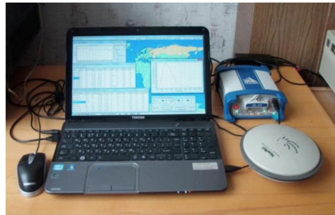
Figure 1. Hardware-software complex of monitoring ionosphere: 1 - navigation receiver, 2 –antenna, 3 - computer, 4 - power adapter, 5 - antenna cable, 6 - interface cable.
